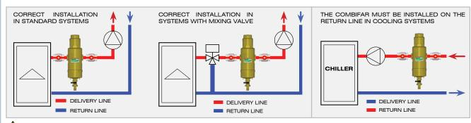
⚠️ Warning! For proper operation the COMBIFAR should always be installed in a vertical position.
