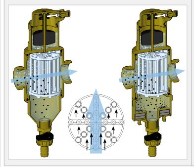
The swiveling COMBIFAR can be installed on the pipeline in either vertical or horizontal position, as the part with threaded connections can rotate 360° around its own axis.
