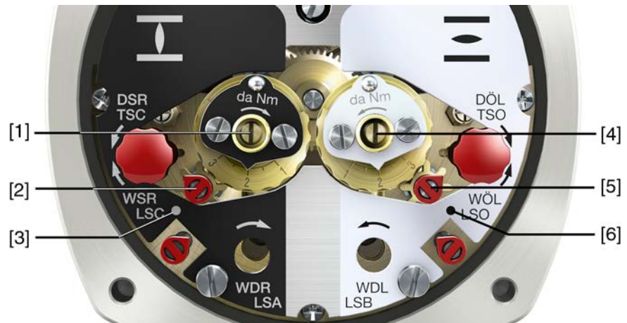
Figure 33: Setting elements for limit switching
