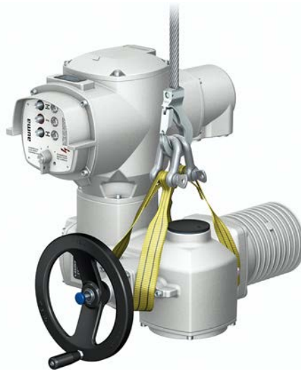
Figure 7: Example: Lifting the actuator
