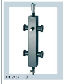
Hydraulic separator complete with automatic air vent valve with non-return valve and drain cock.
