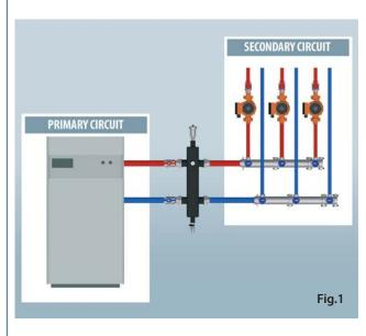
and return circuits, guarding against any kind of interference to either primary or secondary circuit pumps and thus ensuring proper functioning of each and every circuit.
