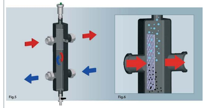
Fig.5 - The illustration shows a section of separator, in which it is The inner mesh, through which the water flows fig.6, permits possible to see the inner mesh. The figure shows also the flow directions under normal connection conditions: i.e. with high temperature supply water in the upper section and with low temperature return water in the lower part.
