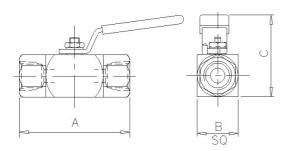
The 'B6' Type Single Isolating Ball Valve is designed for safe and reliable isolation giving bubble tight shut off. Totally enclosed soft seats offer both positive sealing and low operating torques, from vacuum to highpressure service. Anti-blow out spindle is fitted as standard with the option of PTFE or Grafoil seals.
