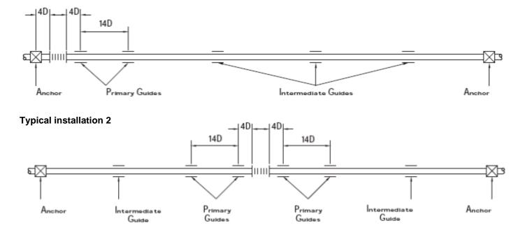
We strongly recommend that this type of slide guide be only used on 80mm nominal bore pipework and below. Please see our type SSHD/SSHDN for further details on pipe slide guides for above 80mm NB pipework.
