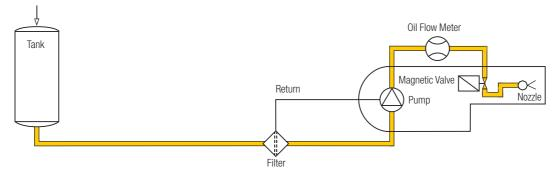
Mounting on suction side of pump (burners)
