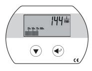
Display values: total volume, resettable volume, flow rate
