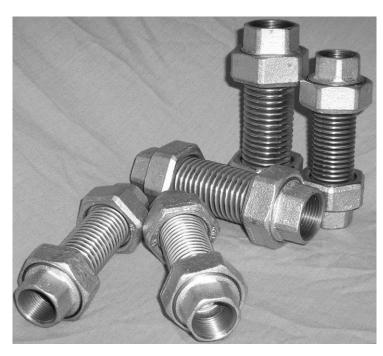
This range of small bore axial expansion joints are specifically designed to absorb the thermal expansion that occurs in hot water and perimeter heating circuits.
